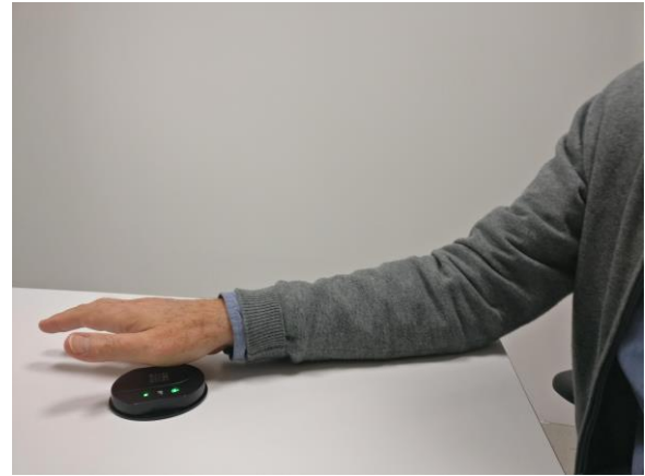
Rest the elbow on the table - no additional force when measuring
